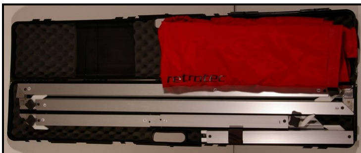
Retrotec Model R43 consists of a DM-2, a 2100 Fan and a cloth door panel.
