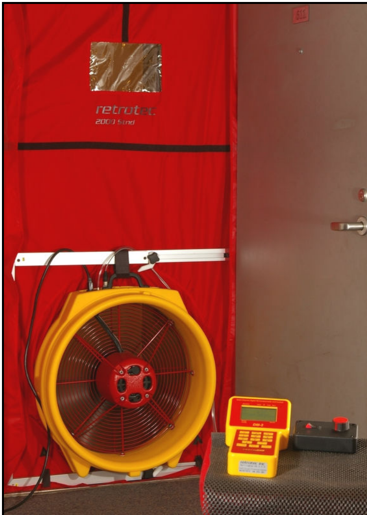
Retrotec Model R43 consists of a DM-2, a 2100 Fan and a cloth door panel.
